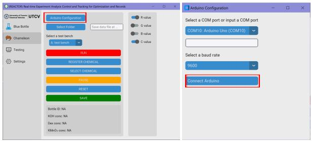
Make sure the correct COM port and correct baud rate (usually 9600) are chosen and then click the 'Connect Arduino' button. The following window should pop up if the connection is successful. Click 'OK' and close the Arduino Configuration window.
